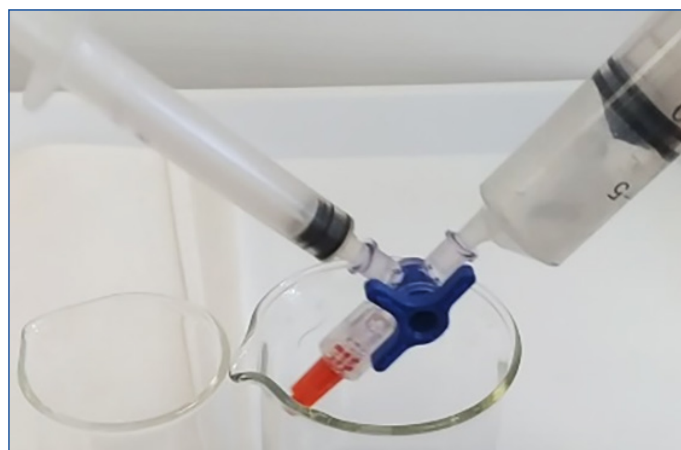
Figure 2 Filling a 2 cm 3 syringe with hydrogen. In this case, the acid is added with a 1 cm 3 syringe on the left.
